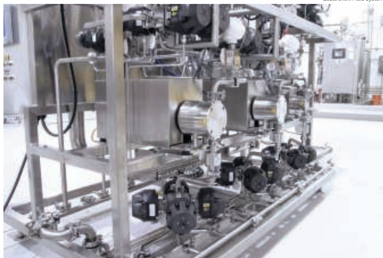
FIGURE 1. Shown here is a chromatography application utilizing three quaternary diaphragm pumps (center, right)
