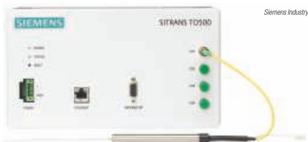
FIGURE 1. The Sitrans TO500 multipoint measuring system evaluates a large number of temperature measuring sensors, which are arranged on a very narrow fiber-optic measuring lance
