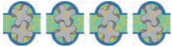
Figure 6. This illustration shows the operating principle of a rotary-lobe vacuum pump [4]
