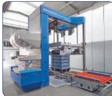
BEUMER stretch hood machines create compact, stable pallet loads
