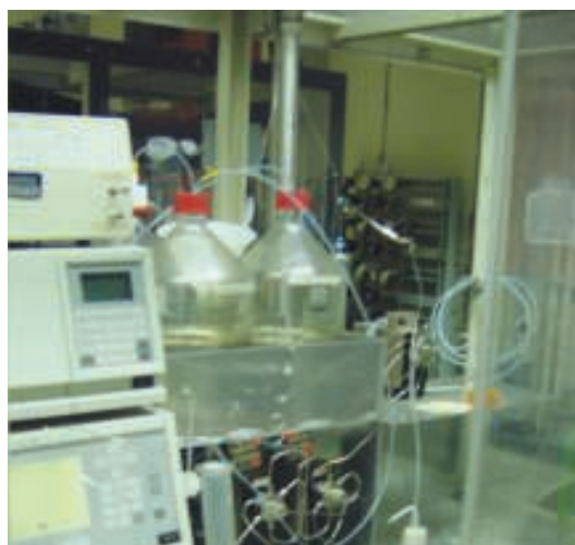
FIGURE 1. The plastic spill-containment basin shown here will not withstand even a small fire
