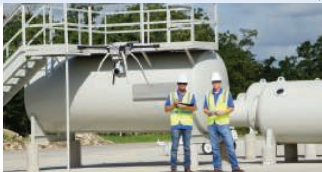
FIGURE 1. Some companies may custom-engineer a drone to carry out specific tasks, such as specialized non-destructive testing or gas detection
