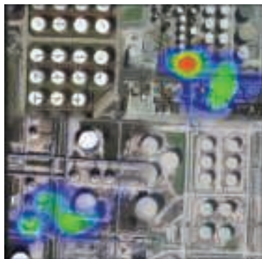
FIGURE 6. Drones outfitted with emissions-monitoring sensors can provide continuous reporting for mapping purposes
