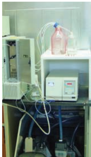
FIGURE 2. Without effective spill containment in place, any spills that might result from these vessels would likely fall to the floor and potentially find an ignition source in the vacuum pump and more fuel in the solvent container located nearby
