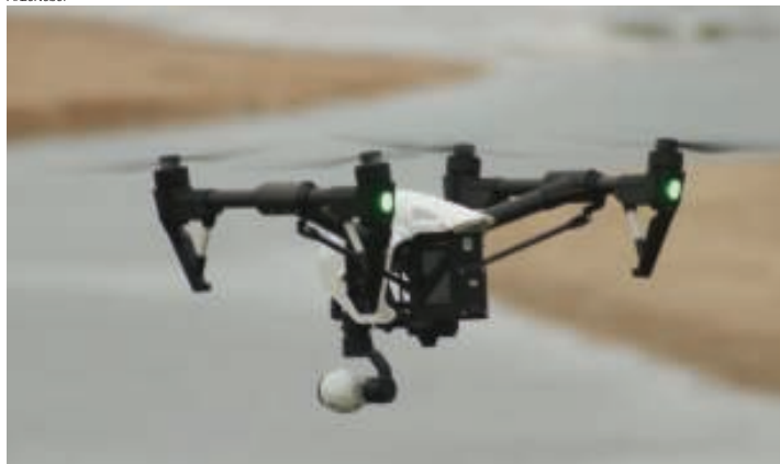
FIGURE 4. Pilot tests are currently underway to commercialize drones for the inspection of coatings in marine environments
